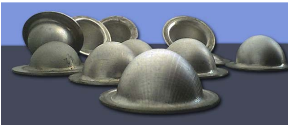
Fig.1 – Gasostatic deep drawing samples
